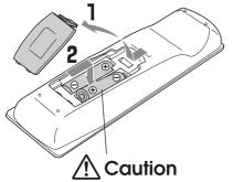
At the time of purchase, the batteries are not inserted into the remote control. Insert the supplied batteries before using the remote control.
