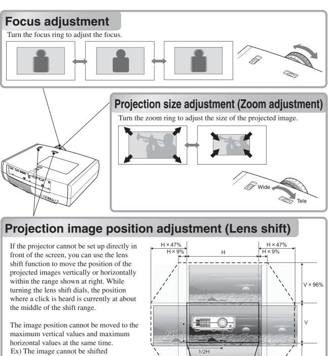
vertically when it has been shifted horizontally by the full amount. When the image has been shifted vertically by the full amount, it can be shifted up to 9% of the horizontal width of the screen.
